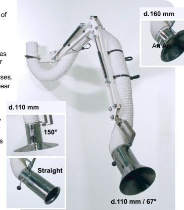
The d.160 mm models are intended for applications where 800-1200 m<sup>3</sup>/h are needed.
