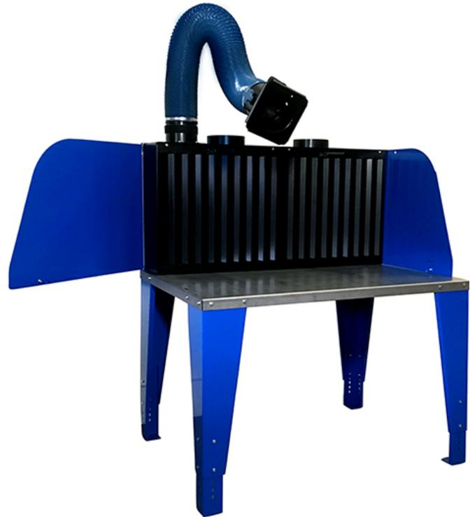
**Extraction Arm.** For heavy welding the Super-Mesa can be equipped with a Flexi FLB 1.5m extraction arm. If it is needed to reach outside the table you can mount a 2m or a 3m Flexi FLB extraction arm.
