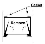
4. Install the new Filter/Filters with GASKET UPWARDS. Turn the exenter BUCKELS UPWARDS.
